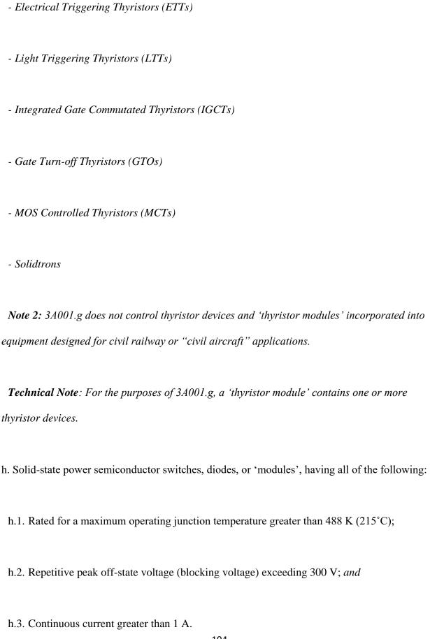
**Technical Note:** For the purposes of 3A001.h, 'modules' contain one or more solid-state power semiconductor switches or diodes.
