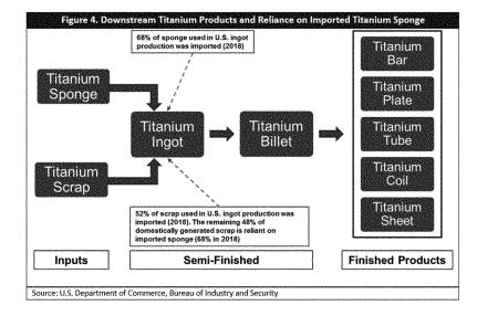
C. Titanium Melting and Finished Titanium Products
