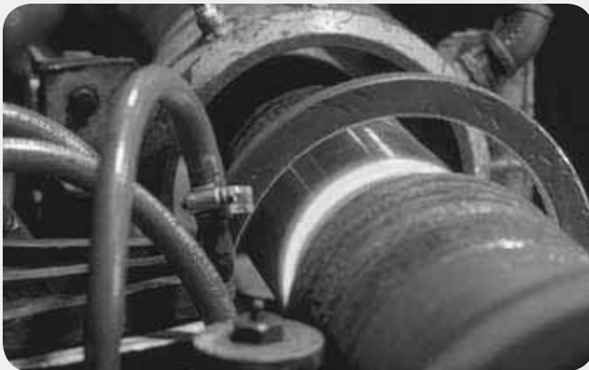
Induction heating and pressurized fluid quench are used in the patented Tuff-Weld® post-weld heat-treating process. The resulting quenched and tempered microstructure maximizes weld area properties.
