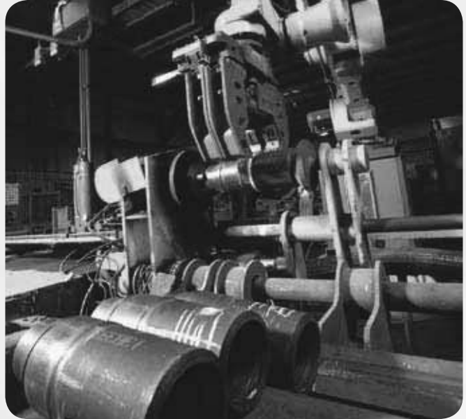
The MTI400VX weld line system is fully automated and features a computerized process, robotic control and laser positioning system.
